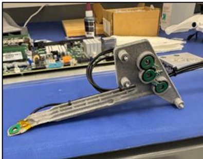
Figure 3: 3D printed sensor harness for accurate and consistency sensor placement.
